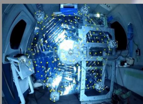
Fig.3 Deployment experiment under micro gravity
