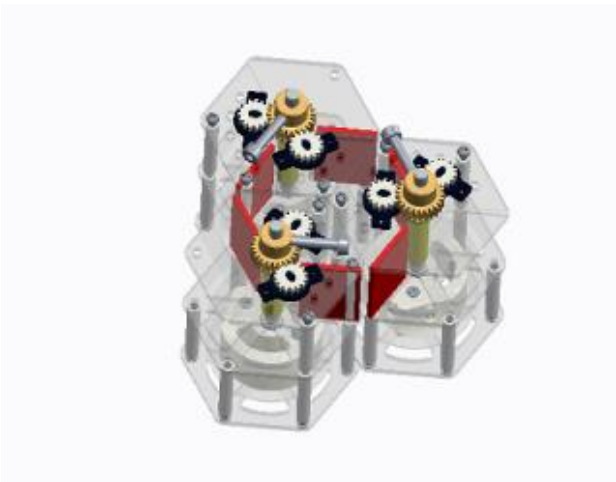
Figure 4(b) Spacer and partition of 3N3B truss model
