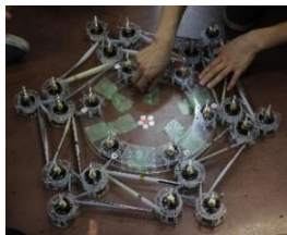
Fig.9 Stored state of 24N42B model (free)
