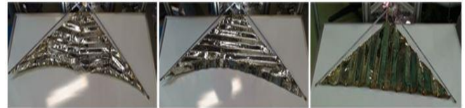
Figure 11 Deployed shape in micro-gravity environment.
