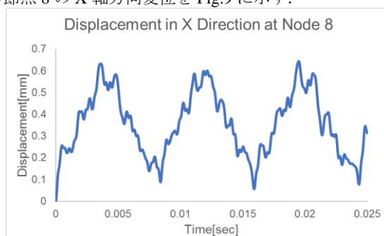
Fig.9 Displacement in X direction in tension at node 8 of flat membrane
